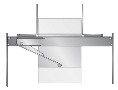
5. Place the removed roll guide back on the roll bar and slide it close to, but not touching, the label stock roll.
